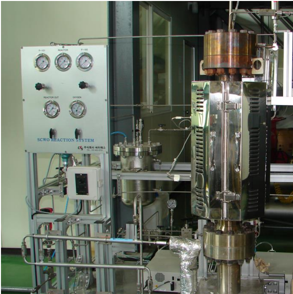
KEPCO SCWO REACTION PILOT PLANT
