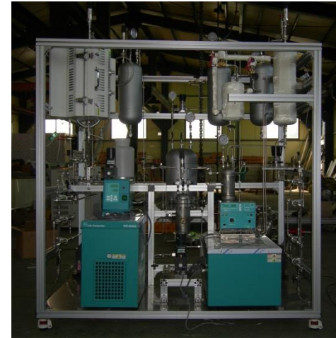
KIER HEAT TRANSPORT PLANT USING METHANOL
